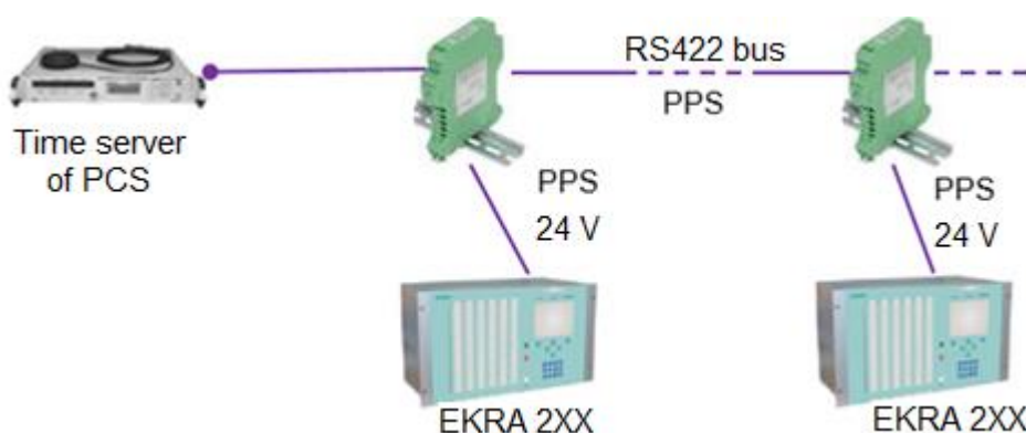
Figure 111 – Standard diagram for connecting the ED2 series device to the time server of PCS via RS422 PPS bus
